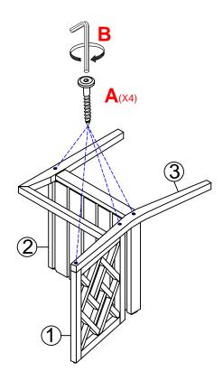
STEP 2: Attach 4 onto 1 and 2 using the screws (A) tighten it up by using an allen key (B)
